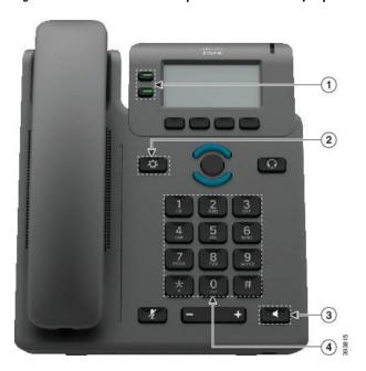
Figure 12: Cisco IP Phone 6821 Multiplatform Phones Mobility-Impaired Accessibility Features
