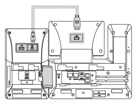
If you connect two expansion modules, connect the USB jack on the prior expansion module and the mini USB jack on the next expansion module using another supplied cable. Connecting two expansion modules on a single host phone is shown as below:
