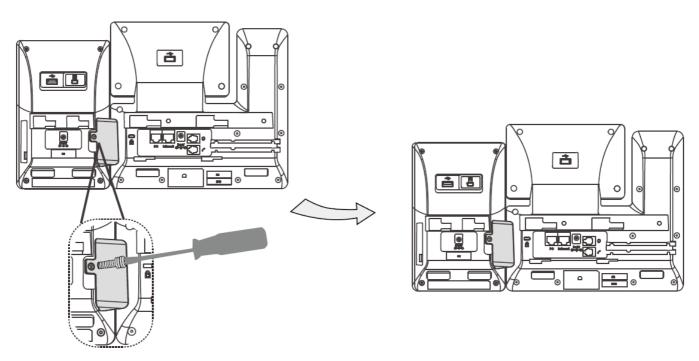
If you want to connect two or more expansion modules, pull out the silica gel and connect two expansion modules as below.
