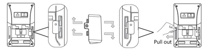
Connecting two expansion modules on a single host phone is shown as below:
