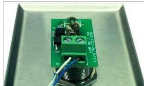
Figure 7: 1203 Call Switch Wiring
