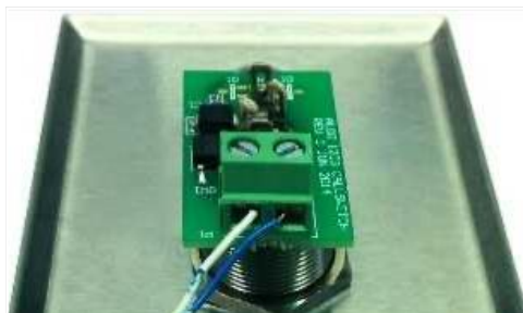
Figure 34: 1203 Call Switch wiring
